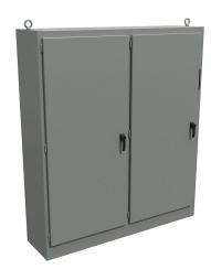
Hammond disconnect enclosure, NEMA 12, right flange, 90 x 79 x 20in (HxWxD), freestanding, carbon steel, ANSI 61 gray, powder coat finish, 2-door, 3-point padlocking handle, subpanel included.
