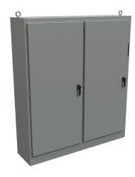
Hammond disconnect enclosure, NEMA 12, right flange, 90 x 79 x 20in (HxWxD), freestanding, carbon steel, ANSI 61 gray, powder coat finish, 2-door, 3-point padlocking handle, subpanel included.
