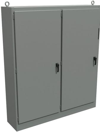
Hammond disconnect enclosure, NEMA 12, right flange, 90 x 79 x 18in (HxWxD), freestanding, carbon steel, ANSI 61 gray, powder coat finish, 2-door, 3-point padlocking handle, subpanel included.
