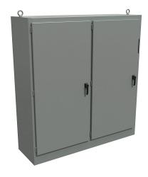
Hammond disconnect enclosure, NEMA 12, right flange, 84 x 79 x 24in (HxWxD), freestanding, carbon steel, ANSI 61 gray, powder coat finish, 2-door, 3-point padlocking handle, subpanel included.
