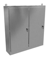
Hammond disconnect enclosure, NEMA 3R/4/4X/12/13, right flange, 84 x 79 x 18in (HxWxD), freestanding, 304 stainless steel, #4 brush finish, 2-door, 3-point padlocking handle, subpanel included.
