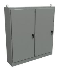
Hammond disconnect enclosure, NEMA 12, right flange, 84 x 79 x 18in (HxWxD), freestanding, carbon steel, ANSI 61 gray, powder coat finish, 2-door, 3-point padlocking handle, subpanel included.
