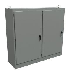
Hammond disconnect enclosure, NEMA 12, right flange, 72 x 79 x 24in (HxWxD), freestanding, carbon steel, ANSI 61 gray, powder coat finish, 2-door, 3-point padlocking handle, subpanel included.
