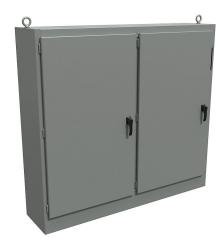
Hammond disconnect enclosure, NEMA 12, right flange, 72 x 79 x 18in (HxWxD), freestanding, carbon steel, ANSI 61 gray, powder coat finish, 2-door, 3-point padlocking handle, subpanel included.
