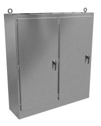
Hammond disconnect enclosure, NEMA 3R/4/4X/12/13, right flange, 72 x 67 x 18in (HxWxD), freestanding, 304 stainless steel, #4 brush finish, 2-door, 3-point padlocking handle, subpanel included.
