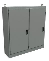
Hammond disconnect enclosure, NEMA 12, right flange, 72 x 67 x 18in (HxWxD), freestanding, carbon steel, ANSI 61 gray, powder coat finish, 2-door, 3-point padlocking handle, subpanel included.
