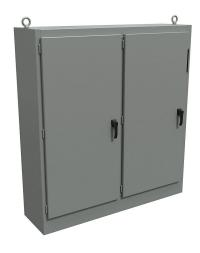
Hammond disconnect enclosure, NEMA 12, right flange, 72 x 67 x 18in (HxWxD), freestanding, carbon steel, ANSI 61 gray, powder coat finish, 2-door, 3-point padlocking handle, subpanel included.
