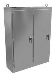
Hammond disconnect enclosure, NEMA 3R/4/4X/12/13, right flange, 72 x 55 x 18in (HxWxD), freestanding, 304 stainless steel, #4 brush finish, 2-door, 3-point padlocking handle, subpanel included.
