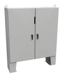
Hammond disconnect enclosure, NEMA 12, center post, 72 x 73 x 18in (HxWxD), floor mount, carbon steel, ANSI 61 gray, powder coat finish, 2-door, 3-point padlocking handle, subpanel included.
