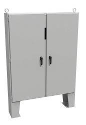
Hammond disconnect enclosure, NEMA 12, center post, 72 x 61 x 12in (HxWxD), floor mount, carbon steel, ANSI 61 gray, powder coat finish, 2-door, 3-point padlocking handle, subpanel included.
