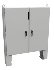
Hammond disconnect enclosure, NEMA 12, center post, 60 x 61 x 12in (HxWxD), floor mount, carbon steel, ANSI 61 gray, powder coat finish, 2-door, 3-point padlocking handle, subpanel included.
