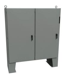
Hammond disconnect enclosure, NEMA 12, right flange, 72 x 74 x 24in (HxWxD), floor mount, carbon steel, ANSI 61 gray, powder coat finish, 2-door, 3-point padlocking handle, subpanel included.
