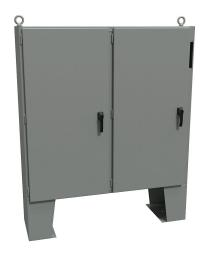
Hammond disconnect enclosure, NEMA 12, right flange, 60 x 62 x 18in (HxWxD), floor mount, carbon steel, ANSI 61 gray, powder coat finish, 2-door, 3-point padlocking handle, subpanel included.
