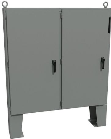
Hammond disconnect enclosure, NEMA 12, right flange, 60 x 62 x 12in (HxWxD), floor mount, carbon steel, ANSI 61 gray, powder coat finish, 2-door, 3-point padlocking handle, subpanel included.
