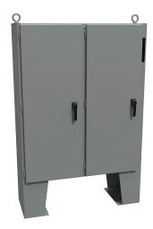
Hammond disconnect enclosure, NEMA 12, right flange, 60 x 50 x 18in (HxWxD), floor mount, carbon steel, ANSI 61 gray, powder coat finish, 2-door, 3-point padlocking handle, subpanel included.
