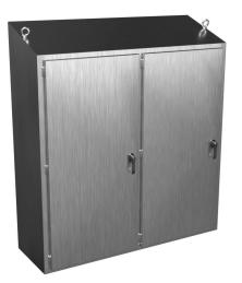
Hammond disconnect enclosure, slope top, NEMA 3R/4/4X/12/13, right flange, 83 x 75 x 25in (HxWxD), freestanding, 304 stainless steel, #4 brush finish, double-door, 3-point 316 stainless steel padlocking handle.
