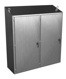
Hammond disconnect enclosure, slope top, NEMA 3R/4/4X/12/13, right flange, 83 x 75 x 25in (HxWxD), freestanding, 316 stainless steel, #4 brush finish, double-door, 3-point 316 stainless steel padlocking handle.
