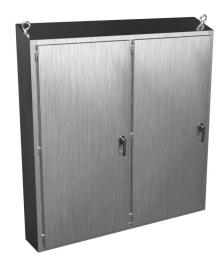
Hammond disconnect enclosure, slope top, NEMA 3R/4/4X/12/13, right flange, 79 x 75 x 13in (HxWxD), freestanding, 304 stainless steel, #4 brush finish, double-door, 3-point 316 stainless steel padlocking handle.
