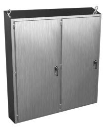
Hammond disconnect enclosure, slope top, NEMA 3R/4/4X/12/13, right flange, 79 x 75 x 13in (HxWxD), freestanding, 304 stainless steel, #4 brush finish, double-door, 3-point 316 stainless steel padlocking handle.
