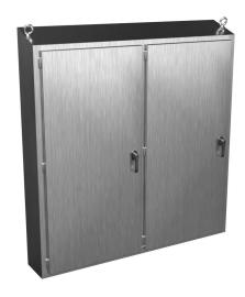
Hammond disconnect enclosure, slope top, NEMA 3R/4/4X/12/13, right flange, 79 x 75 x 13in (HxWxD), freestanding, 316 stainless steel, #4 brush finish, double-door, 3-point 316 stainless steel padlocking handle.
