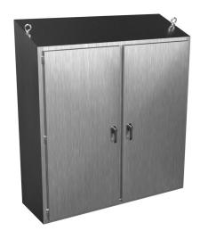
Hammond enclosure, slope top, NEMA 3R/4/4X/12/13, 74 x 75 x 24in (HxWxD), freestanding, 304 stainless steel, #4 brush finish, double-door, 3-point 316 stainless steel padlocking handle.
