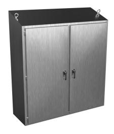
Hammond enclosure, slope top, NEMA 3R/4/4X/12/13, 74 x 75 x 24in (HxWxD), freestanding, 316 stainless steel, #4 brush finish, double-door, 3-point 316 stainless steel padlocking handle.
