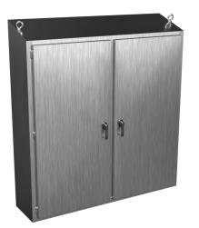
Hammond enclosure, slope top, NEMA 3R/4/4X/12/13, 74 x 75 x 18in (HxWxD), freestanding, 316 stainless steel, #4 brush finish, double-door, 3-point 316 stainless steel padlocking handle.
