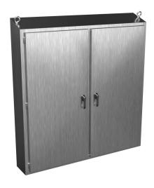
Hammond enclosure, slope top, NEMA 3R/4/4X/12/13,  $74 \times 75 \times 12$  in (HxWxD), freestanding, 304 stainless steel, #4 brush finish, double-door, 3-point 316 stainless steel padlocking handle.
