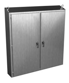
Hammond enclosure, slope top, NEMA 3R/4/4X/12/13, 74 x 75 x 12in (HxWxD), freestanding, 316 stainless steel, #4 brush finish, double-door, 3-point 316 stainless steel padlocking handle.
