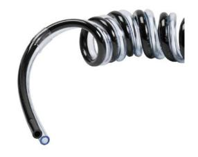
NITRA pneumatic bonded coiled tubing, ether-based polyurethane, black and clear blue, double 5/32in outside diameter, 0.093in inside diameter, 20 coils, 3.5ft (1.07m) working length.
