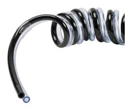
NITRA pneumatic bonded coiled tubing, ether-based polyurethane, black and clear blue, double 5/32in outside diameter, 0.093in inside diameter, 20 coils, 3.5ft (1.07m) working length.
