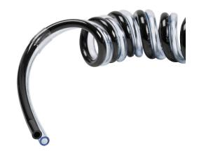
NITRA pneumatic bonded coiled tubing, ether-based polyurethane, black and clear blue, double 5/32in outside diameter, 0.093in inside diameter, 10 coils, 2.0ft (0.61m) working length.
