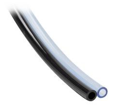
NITRA pneumatic bonded tubing, ether-based polyurethane, black and clear blue, double 5/32in outside diameter, 0.093in inside diameter, 50ft package.
