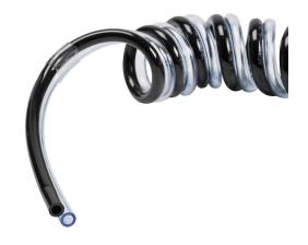
NITRA pneumatic bonded coiled tubing, ether-based polyurethane, black and clear blue, double 3/8in outside diameter, 0.250in inside diameter, 40 coils, 12.9ft (3.93m) working length.
