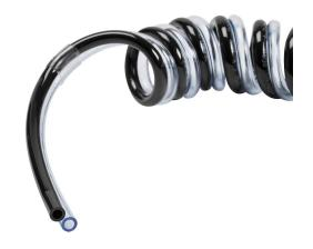
NITRA pneumatic bonded coiled tubing, ether-based polyurethane, black and clear blue, double 3/8in outside diameter, 0.250in inside diameter, 20 coils, 6.7ft (2.04m) working length.
