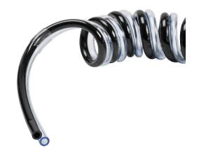
NITRA pneumatic bonded coiled tubing, ether-based polyurethane, black and clear blue, double 1/4in outside diameter, 0.156in inside diameter, 10 coils, 2.9ft (0.88m) working length.
