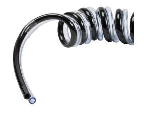
NITRA pneumatic bonded coiled tubing, ether-based polyurethane, black and clear blue, double 10mm outside diameter, 6.5mm inside diameter, 40 coils, 13.0ft (3.96m) working length.
