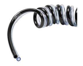
NITRA pneumatic bonded coiled tubing, ether-based polyurethane, black and clear blue, double 10mm outside diameter, 6.5mm inside diameter, 20 coils, 6.7ft (2.05m) working length.
