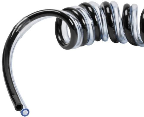
NITRA pneumatic bonded coiled tubing, ether-based polyurethane, black and clear blue, double 8mm outside diameter, 5mm inside diameter, 40 coils, 10.5ft (3.20m) working length.
