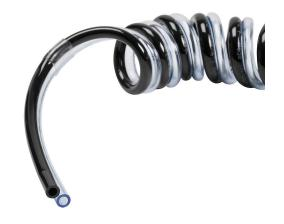
NITRA pneumatic bonded coiled tubing, ether-based polyurethane, black and clear blue, double 8mm outside diameter, 5mm inside diameter, 40 coils, 10.5ft (3.20m) working length.
