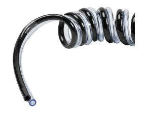
NITRA pneumatic bonded coiled tubing, ether-based polyurethane, black and clear blue, double 8mm outside diameter, 5mm inside diameter, 10 coils, 3.0ft (0.91m) working length.
