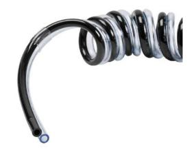
NITRA pneumatic bonded coiled tubing, ether-based polyurethane, black and clear blue, double 6mm outside diameter, 5/32in (4mm) inside diameter, 40 coils, 9.9ft (3.02m) working length.
