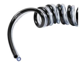
NITRA pneumatic bonded coiled tubing, ether-based polyurethane, black and clear blue, double 6mm outside diameter, 5/32in (4mm) inside diameter, 20 coils, 5.2ft (1.60m) working length.
