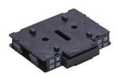
Merz terminal, left or right side mount, 10A @ 600 VAC. For use with Merz ML1, ML2, ML3 Din Rail mount switch bodies -A01, -A02, -E01R, -E02R, -E03R, -E04R, -E05R.
