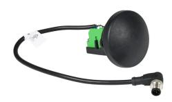
IDEM pushbutton, IP65, 30mm, momentary, (1) N.O./(1) N.C. contact(s), black, mushroom, 68mm, round. For use with IDEM two-hand safety control panels.
