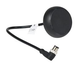
IDEM touch switch, IP65, 30mm, zero force, LED illuminated, (1) N.O./(1) N.C. contact(s), black, mushroom, 68mm, round. For use with IDEM two-hand safety control panels.
