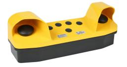
IDEM control panel, two-hand safety, die-cast aluminum, (2) momentary pushbuttons, mushroom, black/black, (1) N.O./(1) N.C. and (1) N.O./(1) N.C. contact(s).
