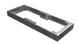
Hammond console plinth,  $4 \times 48 \times 18$ in, 304 stainless steel, #4 brush finish. For use with 2CSC2048 consoles. Field assembly required.
