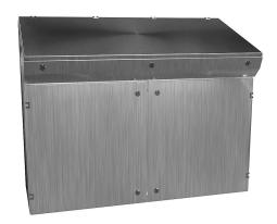
Hammond operator console, NEMA 3R/4/4X/12, 38 x 48 x 20in (HxWxD), freestanding, 304 stainless steel, #4 brush finish, 2-door, 1/4-turn semi-flush oil-tight stainless steel latch.
