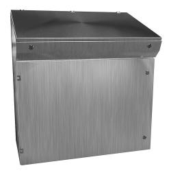
Hammond operator console, NEMA 3R/4/4X/12,  $38 \times 36 \times 20$ in (HxWxD), freestanding, 304 stainless steel, #4 brush finish, singledoor, 1/4-turn semi-flush oil-tight stainless steel latch.
