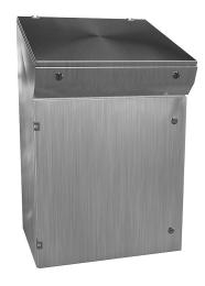
Hammond operator console, NEMA 3R/4/4X/12,  $38 \times 24 \times 20$ in (HxWxD), freestanding, 304 stainless steel, #4 brush finish, singledoor, 1/4-turn semi-flush oil-tight stainless steel latch.
