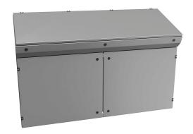
Hammond operator console, NEMA 3R/4/12, 38 x 60 x 20in (HxWxD), freestanding, carbon steel, RAL 7035 light gray, powder coat finish, 2-door, 1/4-turn semi-flush oil-tight latch.
