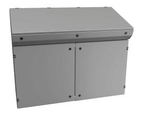
Hammond operator console, NEMA 3R/4/12, 38 x 48 x 20in (HxWxD), freestanding, carbon steel, RAL 7035 light gray, powder coat finish, 2-door, 1/4-turn semi-flush oil-tight latch.
