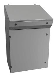
Hammond operator console, NEMA 3R/4/12, 38 x 24 x 20in (HxWxD), freestanding, carbon steel, RAL 7035 light gray, powder coat finish, single-door, 1/4-turn semi-flush oil-tight latch.
