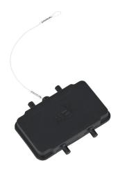
METE cover housing, 4-peg, connector housing size 10B, heavy-duty thermoplastic. For use with METE size 10B double lever connector housings.
